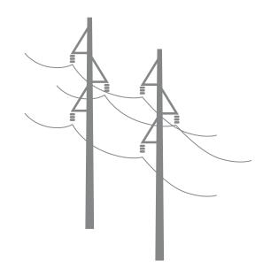
SWEPCO typically uses 69 kV, 138 kV and 161 kV transmission lines to move power shorter distances -for example, to different parts of a city or county.
